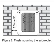
Figure 2. Flush mounting the subwoofer. Note the clearance needed on the reflex port side.
